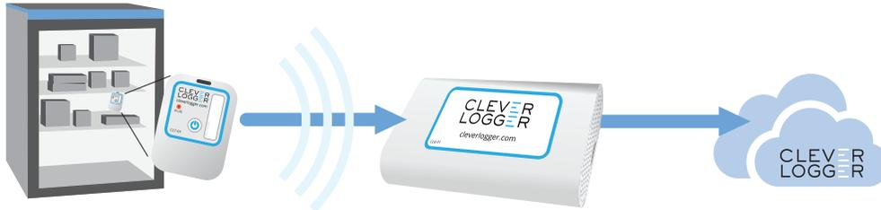
The **logger** measures the temperature and wirelessly sends the reading to the gateway. No need to manually download data.
